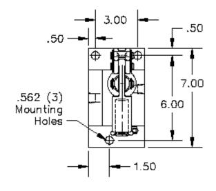
Star Hydraulics, LLC Series CPS-LR Hand Pump Two Speed, Base Mount, Screw Release No Reservoir.
