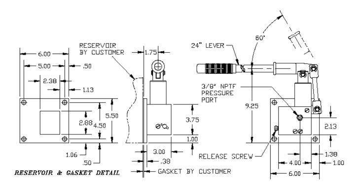
Star Hydraulics, LLC Series CPS-PL Hand Pump Two Speed, Flange Mount, Screw Release
