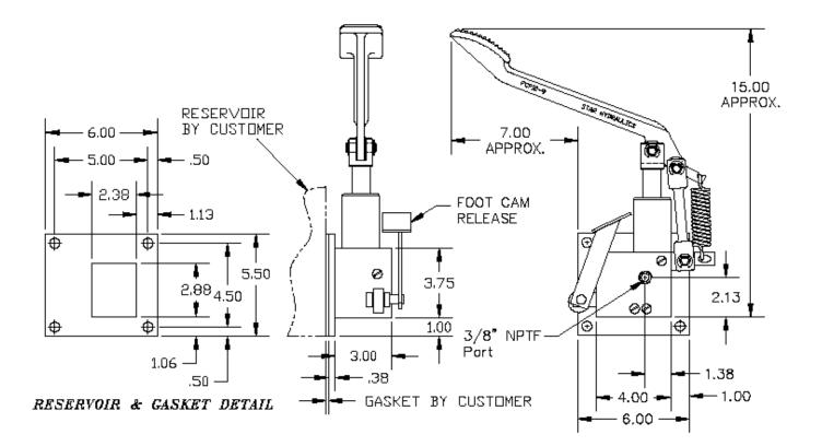
Star Hydraulics, LLC Series FCP-PL Foot Pump Two Speed, Flange Mount, Foot Cam Release
