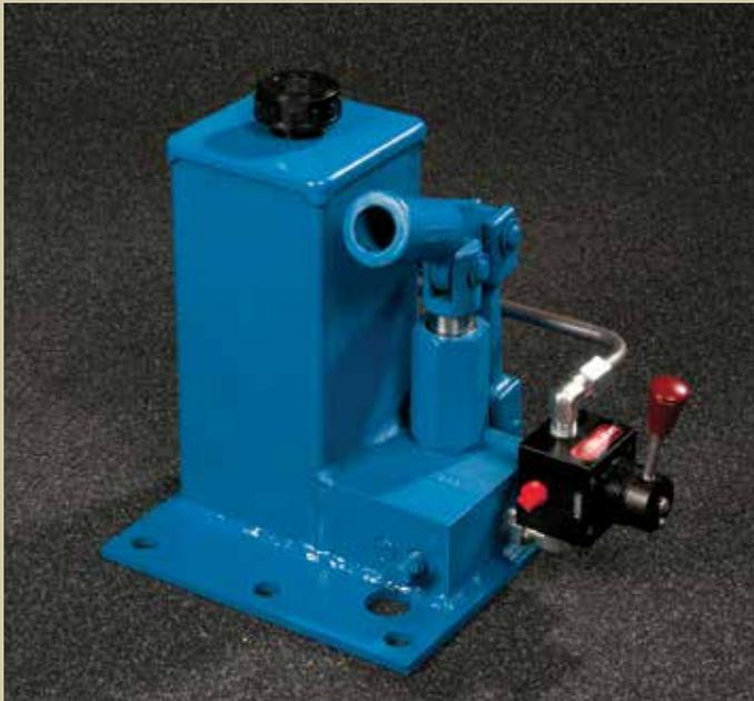
**Pumps with 4-way valves** are used with double-acting cylinders. This 4-way valve allows the pump to advance or retract a double-acting cylinder at full pump pressure.
