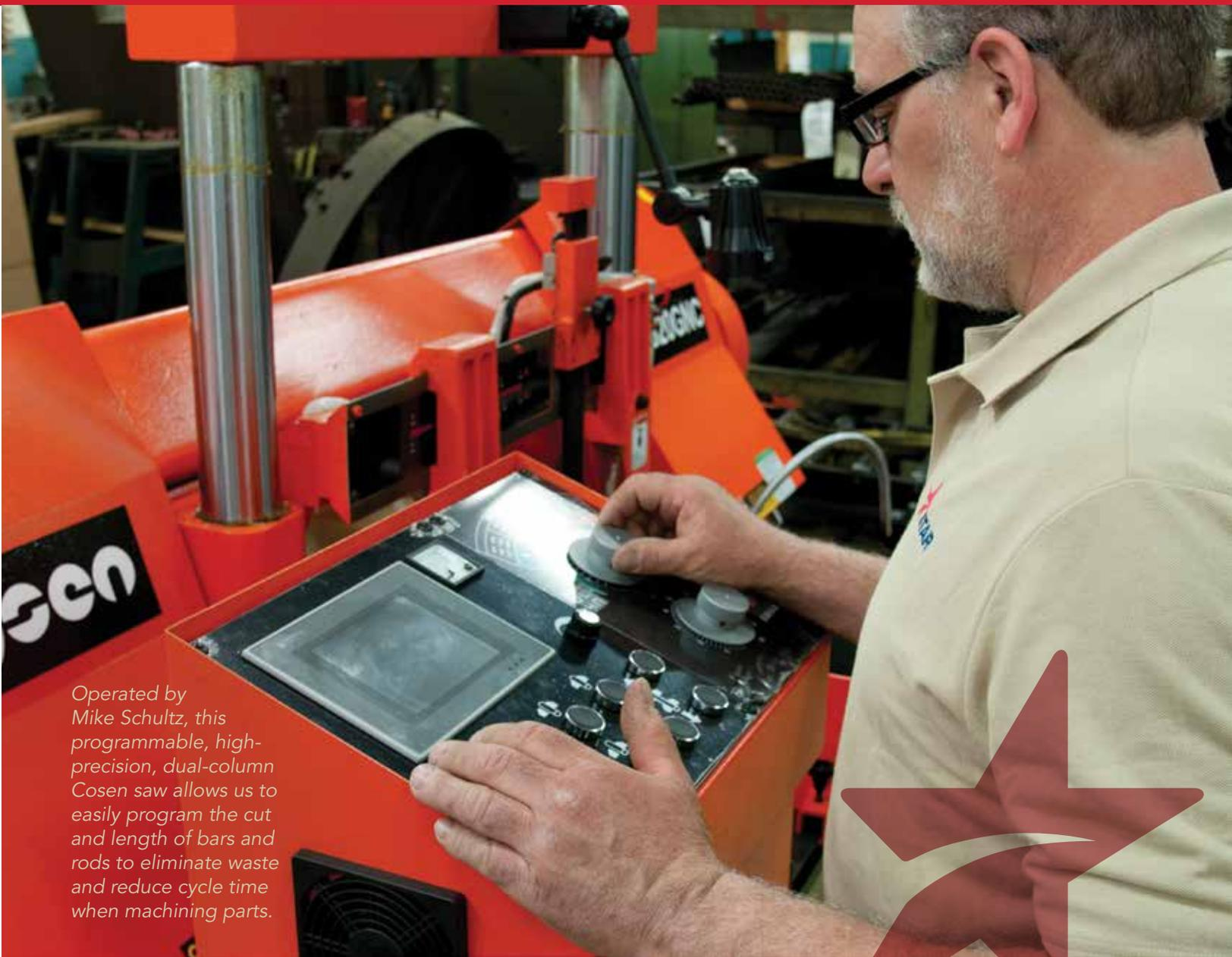
*Operated by Mike Schultz, this programmable, high-precision, dual-column Cosen saw allows us to easily program the cut and length of bars and rods to eliminate waste and reduce cycle time when machining parts.*
