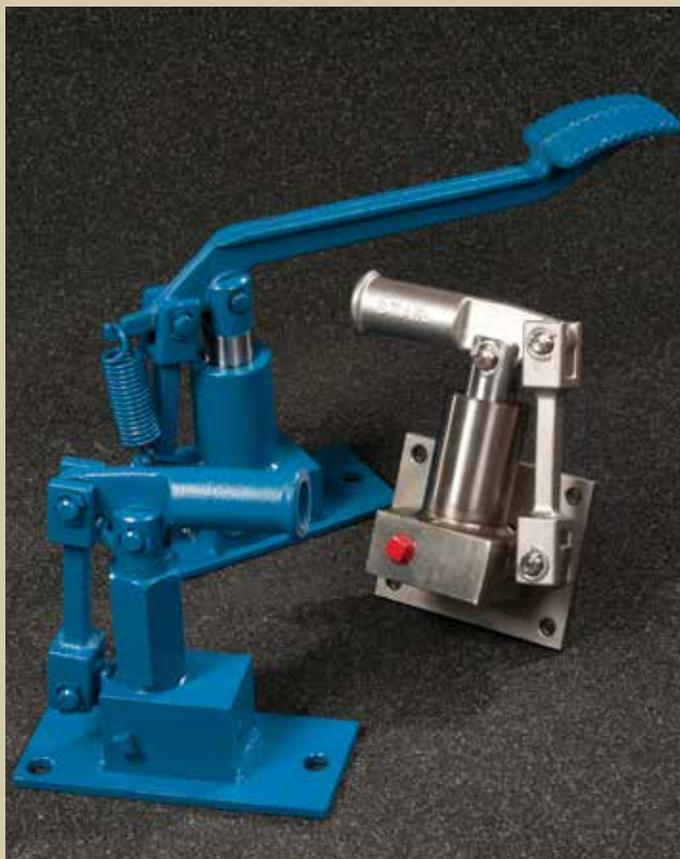
**Our Star simple pump** is a low-cost, efficient means to develop or increase pressure in a hydraulic system. This is a basic pump with no reservoir, overload relief valve or release valve; it is meant for use in a hydraulic system with its own reservoir and control valves. In emergencies, it supplies reliable hydraulic power to operate presses, valves, doors and safety locks, or cylinders that actuate other devices.
