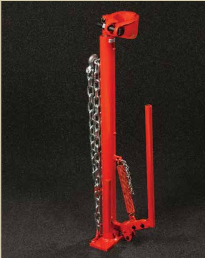
One person can operate this compact, lightweight, **portable post straightener** with 1-ton lifting capacity to straighten concrete-mounted pipes and posts up to 2 in. thick. Our heavy-duty model has a 2-ton lifting capacity and can straighten posts made of 2½ in. pipe. These tools are designed for straightening parking meter posts, sign posts, fence posts and other posts made of heavy-duty pipe. One person can easily straighten a post in just a few minutes.
