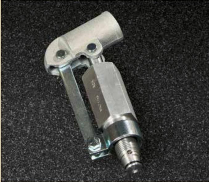
**Star manifold-mounted hand pumps** provide a low-cost, efficient means to manually develop or increase pressure in a hydraulic system. Use it as a primary pump for a hydraulic system or a standby pump for emergencies. It operates presses, valves, doors, safety locks and other devices. This manifold pump is complete with suction and pressure check valves. Designed to mount directly in your manifold block, it eliminates the need for a costly valve body.
