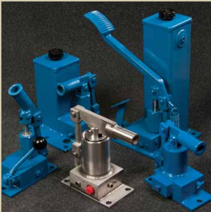
These **single-piston pumps** are solid, heavy-duty, versatile manual pumps with built-in reservoir. P Series pumps include both adjustable overload valves and pressure relief valves. The standard model provides a simple screw pressure release valve for controlled lowering speed. Or save time and reduce pressure with an easy-to-use cam pressure release valve. Options include foot-activated models, stainless steel versions and 4-way valve models.
