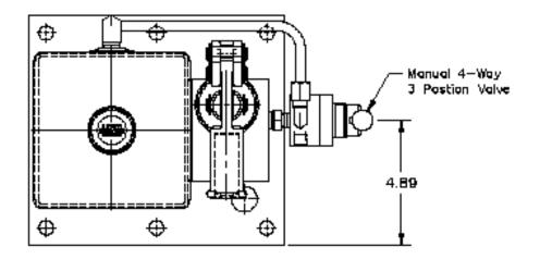
Star Hydraulics, LLC CP series hand operated pump with 4 way valve.
