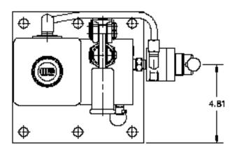
Star Hydraulics, LLC P series hand operated pump with 4 way valve.
