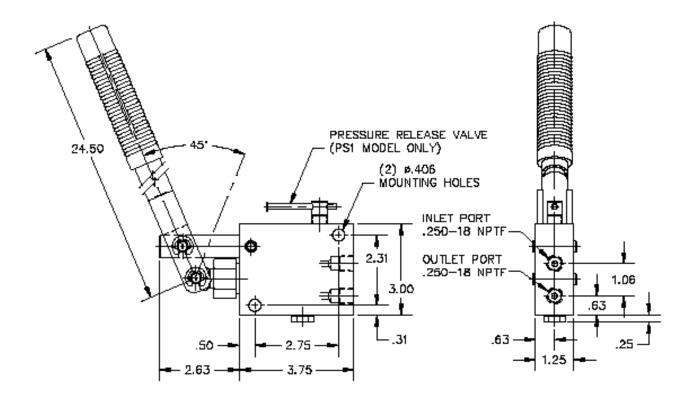
Star Hydraulics, LLC Single Speed Manual Hand Pump Model PS1
