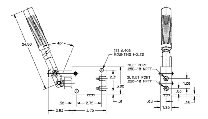
Star Hydraulics, LLC Single Speed Manual Hand Pump Model PS2 Maximum Pressure: 5,000 PSI Volume per Stroke: .3 cu. In. Handle Force per 1,000 PSI: 19 Lbs. Net Weight: 6 Lbs.
