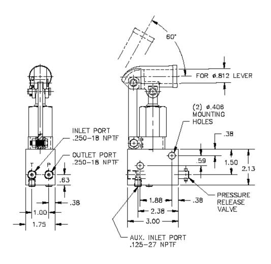
Star Hydraulics, LLC Single Speed Manual Hand Pump Model MK1930
