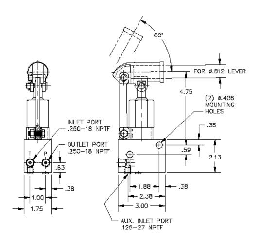
Star Hydraulics, LLC Single Speed Manual Hand Pump Model MK1930-LR (No Release) Maximum pressure rating: 2800 PSI
